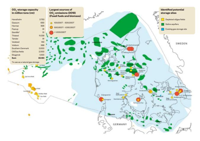
In Denmark, the primary storage locations for  $CO_2$  are anticipated to be porous and permeable sandstone layers, covered by one or more layers of sealing claystone. There are several different storage options available in Denmark, which should be examined to ensure that the right solutions are chosen on a national basis:
